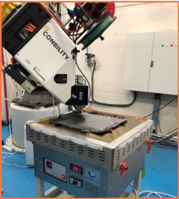
AFP/ATL laminate being consolidated on a heated layup tool © AIMEN
