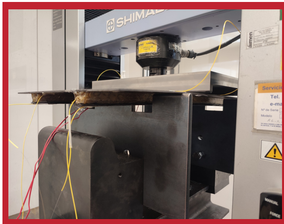
Figure 3: DOMMINIO stiffened panel tested according to Four Point Bending based on ASTM D6272
