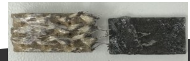
Disassembled gyroid stiffener from CF/LM PAEK laminate using localized induction heating
